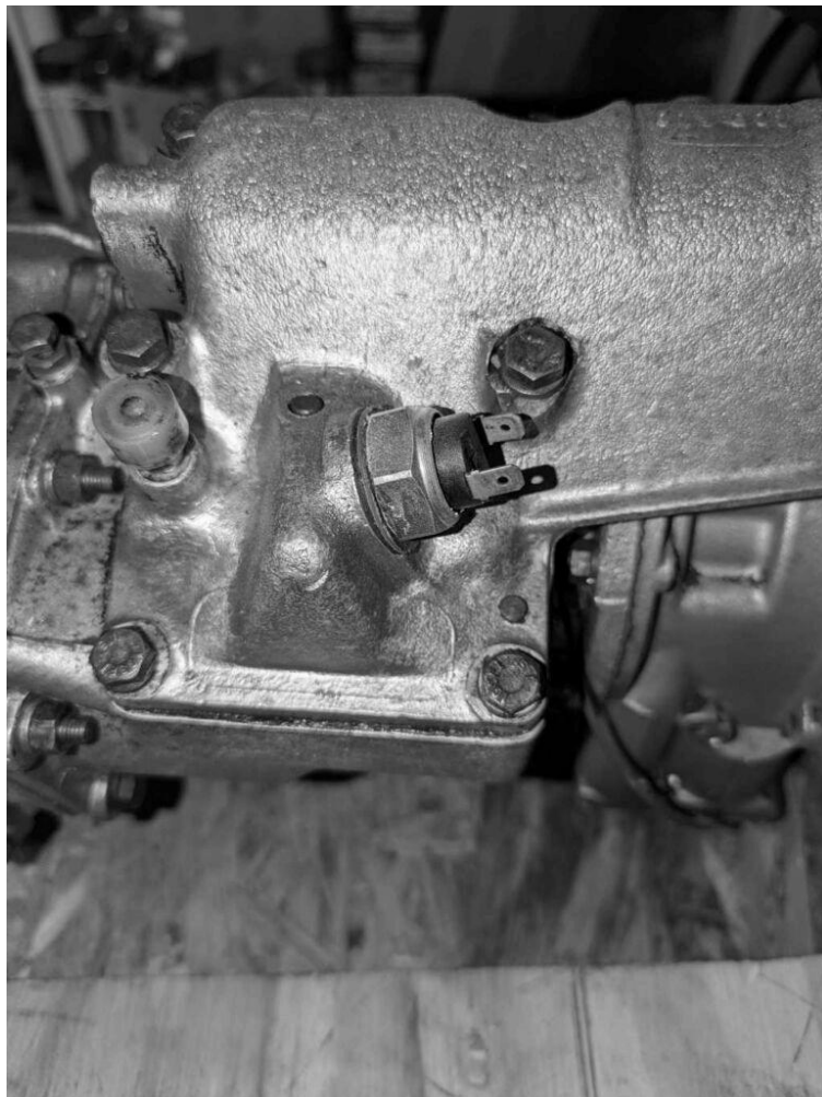
Closeup of the Transmission Interlock Switch (TIS)
