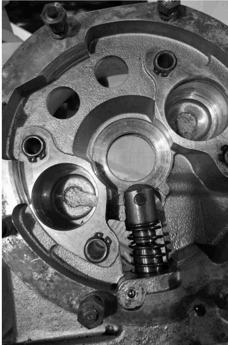
Image of the oil pump installed in the overdrive adapter
