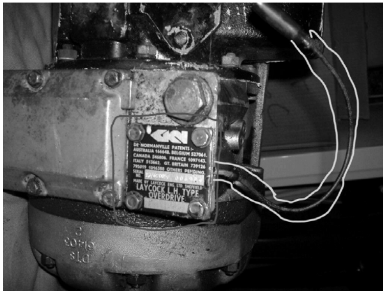
Red box is the solenoid cover plate. Yellow is the power wire
