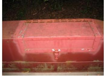
But, there is a solution. Cut out a portion of the left hand fender top and inside so that you can open the car door. The positioning and size of this hinged flap will vary from trailer to trailer. When in use, place a towel over the opening to protect the car's door!
